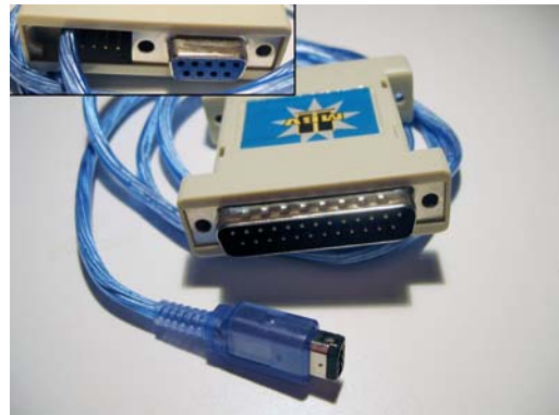
Illustration 3.2.7 - A "Multi-Boot v2" cable
